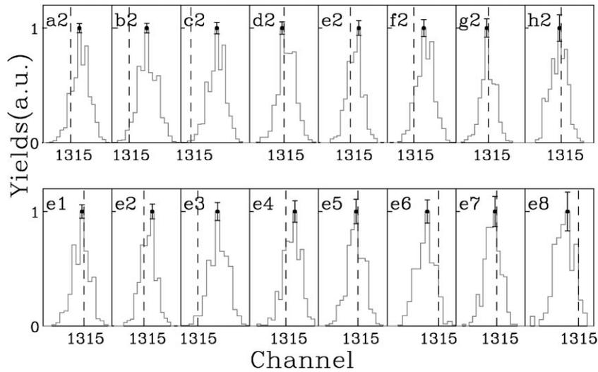
Fig. 5. Energy spectra of 240 MeV  $^4\text{He}$  particles for individual pixels. The upper panel shows 8 spectra down column “2” and the lower panel shows eight spectra across Row “e”. See Fig. 4 captions for explanation of pixel identification.
