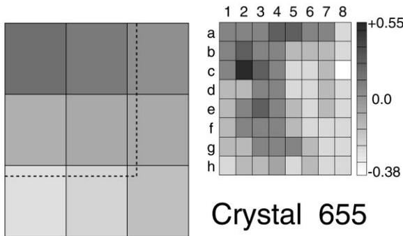
Fig. 4. Variations in light output from the scanning of 5.486 MeV alpha particles (left panel) and from 240 MeV  $^4\text{He}$  particles pixel by pixel (right panel). The  $8 \times 8$  pixel shaded area in the right panel corresponds to the area enclosed by the dashed line in the left panel. Column numbers (1–8) and row letters (a – h), used to identify each pixel in Fig. 5, are marked.
