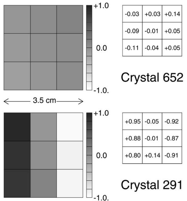
Fig. 1. Results of alpha source scans for two crystals. The non-uniformity gradient in Crystal # 652 (top panel) is less than  $\pm 0.5\%$  and was accepted. However, the scanning results for Crystal # 291 (bottom panel) is outside  $\pm 0.5\%$  non-uniformity and was rejected.
