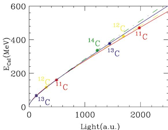
Fig. 7. Calibration curves for  $^{11}\text{C}$ ,  $^{12}\text{C}$ ,  $^{13}\text{C}$  and  $^{14}\text{C}$  for the CsI (Tl) crystals obtained using direct fragmentation beams listed in Table 1. The curves are the best fit according to Eq. (2).
